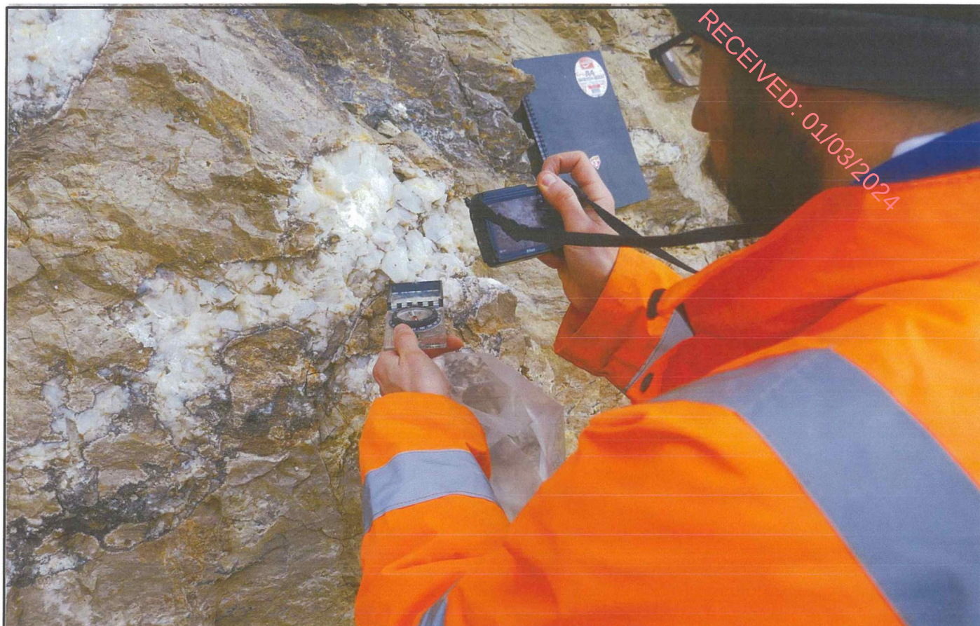
Figure 2.22 Rathcore Quarry - geological and structural mapping of exposures
